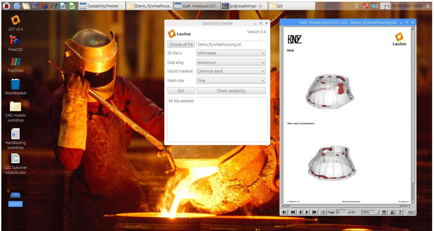
Lautus Castability Checker (LCC) is a clever tool to calculate the castability of a CAD design. Handling is remarkably easy. Anyone can use it without training. The pre-processor and the postprocessor work fully automatically. The compact hardware makes it *plug-and-play* on each location.
