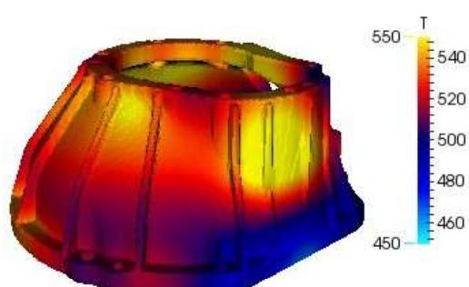
Temperatures at 10%, 25%, 50%, 75%, 90% and 100% of the solid fraction.
